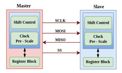
The SPI function core consists of four main modules: SPI interface, SPI master module, SPI slave module, SPI top module.
