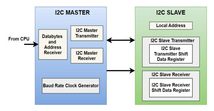
The I2C Protocol core consists of 2 modules: I2C Master , I2C Slave.
